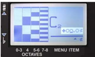
4. To change the value of the displayed parameter, rotate the "Value" knob.
