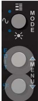
2. To step through the parameters of each device, press either of the two "Menu" buttons below the "Mode" button.
